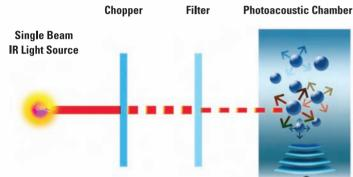
Photoacoustic IR (PIR) directly measures pressure changes caused by IR light absorption. The higher the pressure, the greater the concentration of measured gas.
